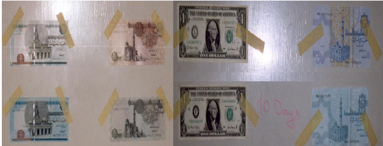
Figure "6": The Egyptian banknotes & the USDs, after (10 days) chloroform bleeding
