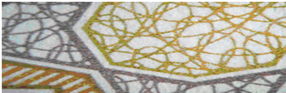
Figure "7": The brown & yellow dry offset printed lines on the Egyptian 1 pound Banknote
