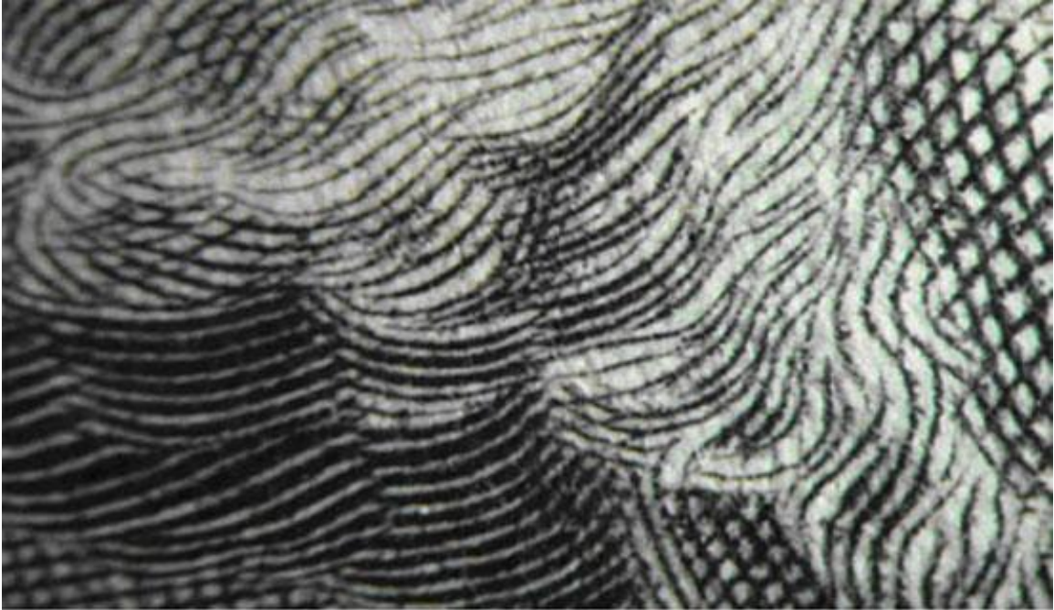
Figure "4": The original embossing rough intaglio printed lines on the 1 USD banknote
