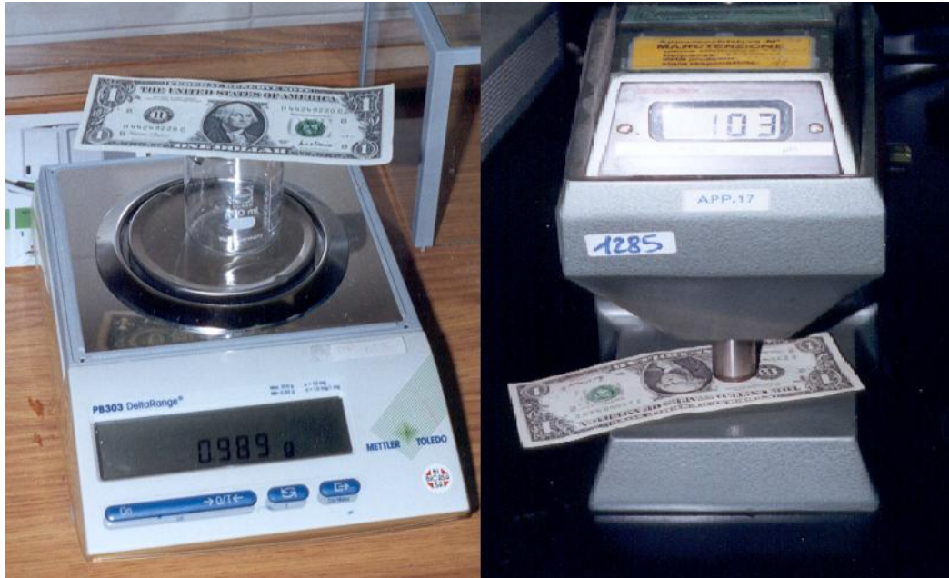
Figure "1": Measuring the USD basis weight (left) & thickness (right)
