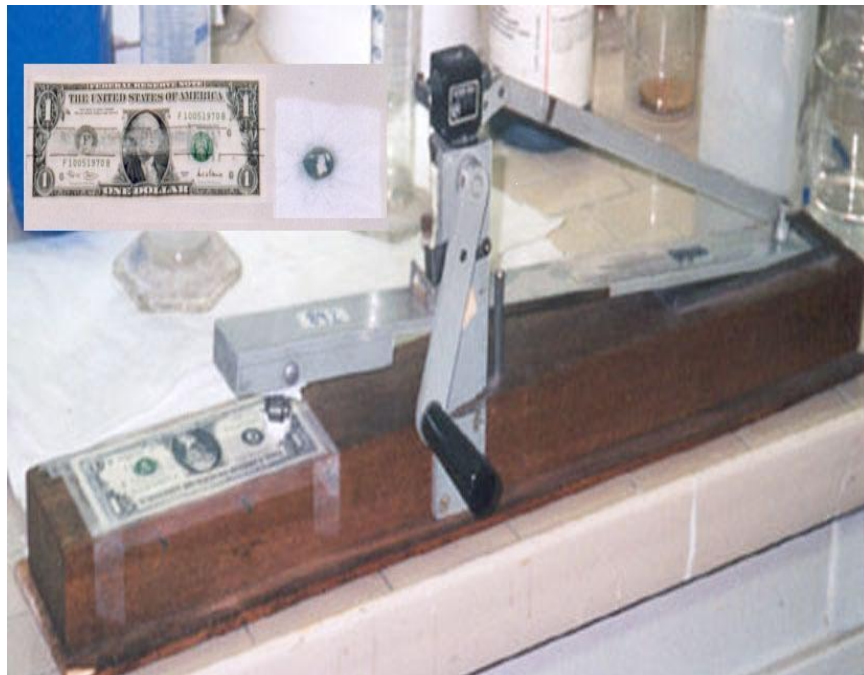
Figure "3": The cotton covered plastic rub head on the 1 USD banknote
